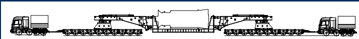
Heavy duty tractors, 2x10 heavy-load axles with Schnabel trailer and generator in a low-bed
